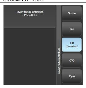
You can change the invert on multiple fixtures by selecting more than one, but the "Inverted" display will not show if there is a mixture of inverted and non-inverted fixtures in the selection.
