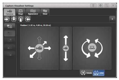
The left hand pad moves the camera left and right, and towards and away from the stage.
