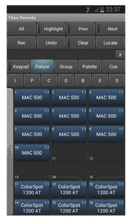
You can then use the Palette screens to control the fixtures, or press the IPCGBES buttons to directly control functions of the fixtures using wheels.
