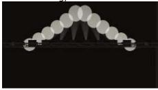
Pull Ends - The first and last selected fixture are affected most, the midpoint is unchanged. This is useful for colour mixing, tilt and dimmer.
