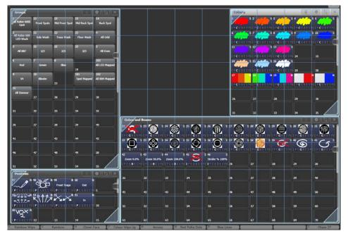
To set one of the standard sizes, open the Window Appearance menu using the Cog button at the top of the screen. Some consoles also have hardware buttons for Min/Max (toggle the window between full and quarter size) and Size/Position (move the window around the possible positions and screens).
