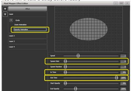
6> Click on [Effect] again and reduce 'Master Speed' to your preference. (Adjusting the global speed control ensures the zoom and opacity animations are synchronised instead of
