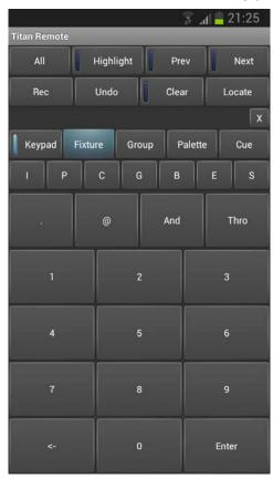
The User Number of the fixture or dimmer is used for control. For example to turn on dimmer 3 at 50% you would press:
