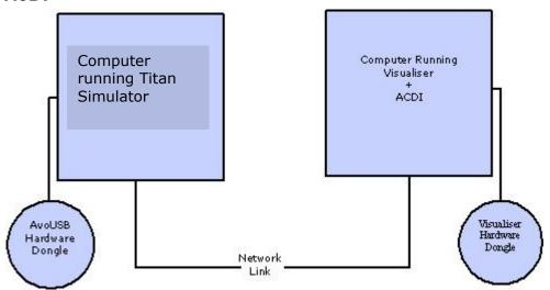
The network link connection can be made through either a crossover cable, or through a network hub.
