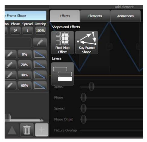
You can also add a completely separate key frame shape or a pixel map effect. Pixel map effects will be shown at the top of the shape list on the left, you can use the eye icon to hide the pixel map effect when you want to work on the key frame shapes.
