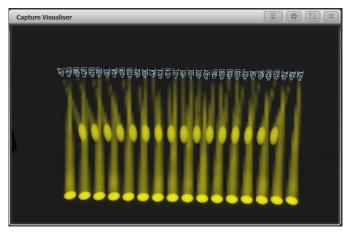
The display above the left hand wheel shows the phase in degrees. For example, 180 degrees repeats every 2 fixtures, 90 degrees repeats every 4 fixtures, 60 degrees repeats every 6 fixtures, and so on.
