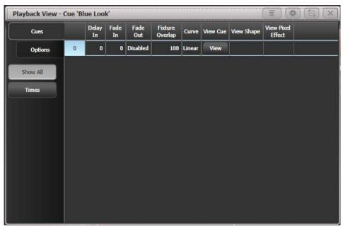
You can configure which columns are shown in the Playback View using the [Edit Columns] context menu button. Once you have set a view you can save it to a filter button which appears below the Times button on the left.
