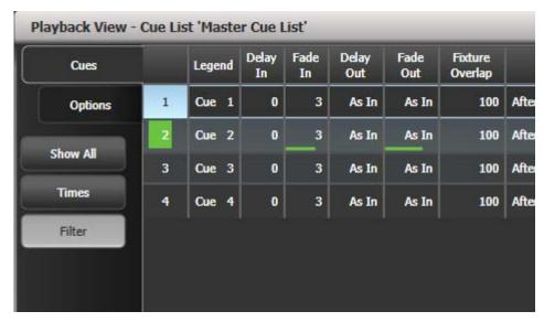
When times are in progress on a cue, green progress bars are shown in the Playback View window.
