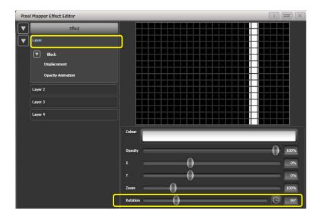
Now you have a vertical bar that draws randomly using a horizontal displacement. Similarly you can use the [layer] or [effect] controls to make global changes to X/Y position and Zoom allowing quick manipulation of entire effects.
