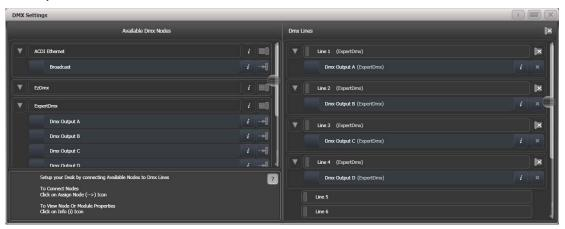
You can individually assign Nodes to Lines using the arrow button, or assign all Nodes of the same type using the group assign button. For example, to assign each XLR output socket on the back of the console to a DMX line, you would click on the Group Assign button of the ExpertDMX nodes.
