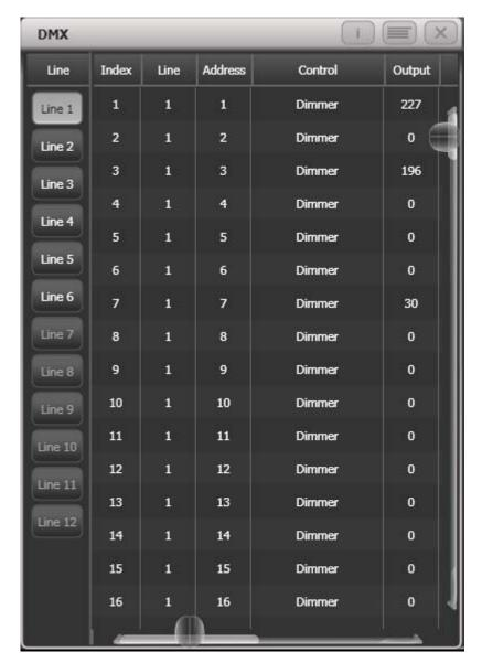
The buttons on the left let you select the different output lines from the console. Scrolling the window to the right shows more information about each DMX channel.
