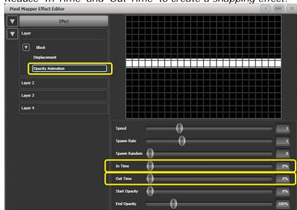
Reduce 'In Time' and 'Out Time' to create a snapping effect.
