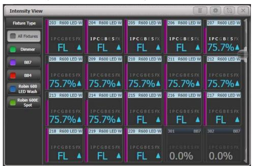
Each fixture has a block showing the intensity as a number and as a bar down the left side. The header bar shows selection/programmer state like fixture buttons – blue for selected and cyan for in programmer.
