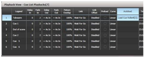
The Autoloaded playback will be fired when the cue starts, and killed when the cue list moves on to the next cue, unless you have also loaded the playback into the next cue.
