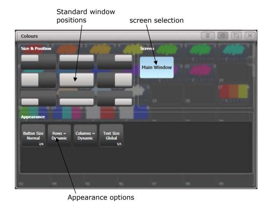
As well as the standard window sizes, you can set custom window sizes and positions using the **Window Layout** button. See section 13.2.2 on page 234 for details.
