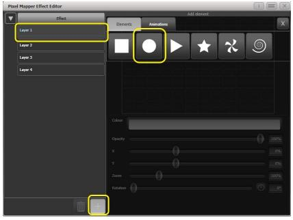
7> Drag the 'Zoom' slider until the circle covers approximately one cell. You can also use the 'Width' and 'Height' sliders to turn the circle into an oval if that helps.
