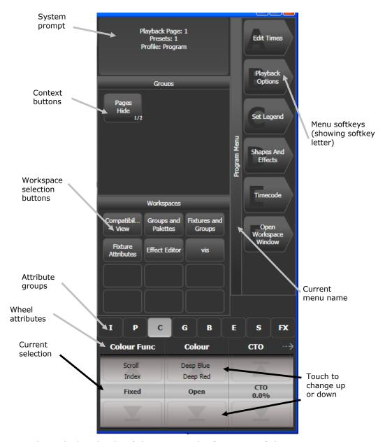
Down the right hand side of the screen, the functions of the A-G menu softkeys are listed. If there are more functions than will fit on one screen, [Previous] and [Next] buttons are provided to page through the functions. You can either press the real button next to the screen or touch the key on screen.
