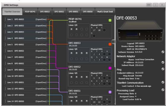
The left side of the screen shows the 64 possible DMX output lines on the console. To the right of this are the processing nodes which are connected, the top one being the console itself. Each node shows how the lines are allocated to the physical outputs on the device. Clicking this area will open the detail tab for the node.
