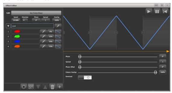
The controls at the top of the left hand pane are the global shape properties which affect the whole shape, controlling speed, direction (using 2D group layout), phase/spread and fixture overlap. The eye icon in the top left corner "collapses" the shape preview in the effect editor window, this allows you to expand only the shape you want to work on if you have created multiple shapes.
