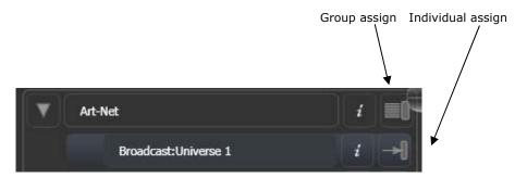
To assign a node to a line, click on the arrow on the node (the node will be highlighted), then click the line you want to assign to it.
