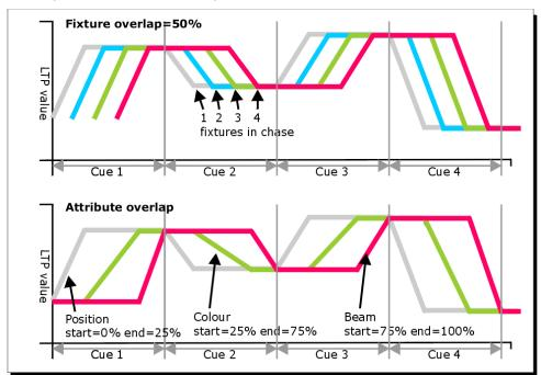
• Press [Fixture Overlap] then enter 0-100 on the keypad to change how fixtures overlap in the cue. 100% (the normal setting) means all fixtures fade together. 0% means that the first fixture will finish its fade before the next one starts giving a "rolling" change across a range of fixtures. 50% means that the 2<sup>nd</sup> fixture will start fading when the first one is half way
