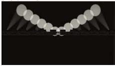
Arrow - The first and last selected fixture are affected equally to the midpoint fixture but in the opposite direction. This is useful for colour mixing, tilt and dimmer
