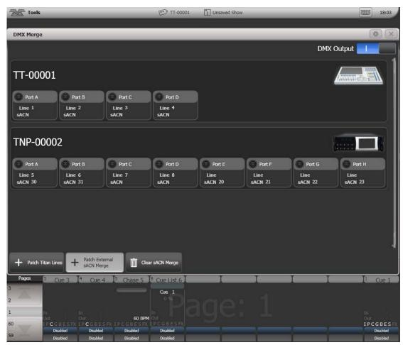
To configure an output port, click on Patch Titan Lines, enter universe number then click on a port to assign.
