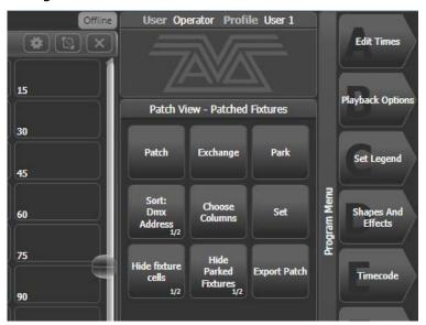
The **Window Appearance Options** button (cog icon) lets you select the standard window sizes and positions. Buttons are also shown allowing you to set the button size and the text size of the window. The Appearance options may vary depending on which window it is, the setup of the console and if you have any external monitors.
