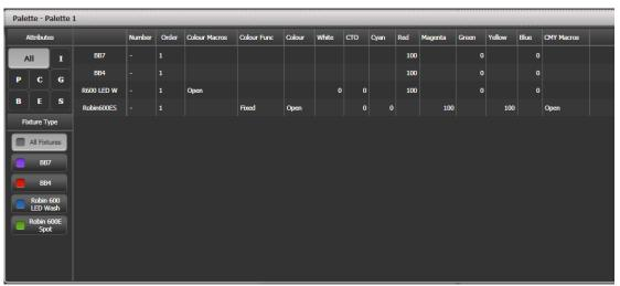
You can filter which attributes are shown using the All/IPCGBES buttons in the top corner, or which fixtures are shown using the fixture type buttons below that.
