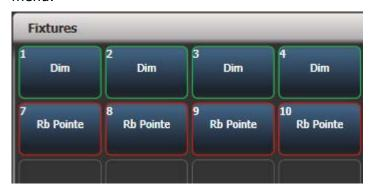
If you set a halo on fixture buttons, the halo colour is also used in other windows; fixture buttons can also have an automatic halo to help identify different types of fixture. There is more information on fixture halos in section 3.2.6 on page 60.
