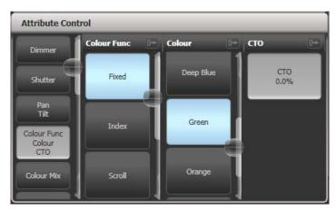
The rest of the window contains buttons or controls to set the attribute value. For attributes such as gobos and fixed colours, a button is provided for each one, making selection a lot quicker than scrolling through on a wheel.
