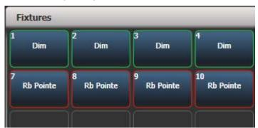
To enable automatic halo colours, hold Avo and select [User Settings], then [Handles], then set Fixture Halos to [Auto]. Fixture buttons will then be coloured to match the automatic fixture colours used in the Patch window.
