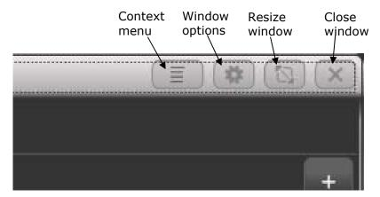
The **Context Menu** button is only shown on Sapphire Touch and Titan One, and gives a drop down menu at the top of the window showing the context menu buttons which relate to the current window.
