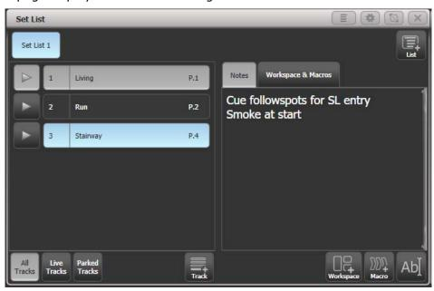
A set list is made up of tracks. When a track is added it automatically links to the current page. Pressing the play button next to the track will automatically select the correct playback page (except on Pearl Expert, because the rollers cannot be moved automatically).
