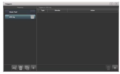
The left hand side of the window has a list of trigger sets. The "classic Pearl" MIDI trigger implementation is provided as one of these. Each set of triggers can be enabled or disabled using the button at the right hand end of the mapping name.
