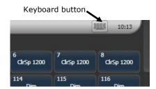
The touch keyboard can be switched between large and small size using the Max/Min button and you close it using the large X button in the top right hand corner. It can be set to pop up automatically when text input is required, using the Man/Auto button. You can also move it on the screen by touching and dragging the blank area of the keyboard at the top.
