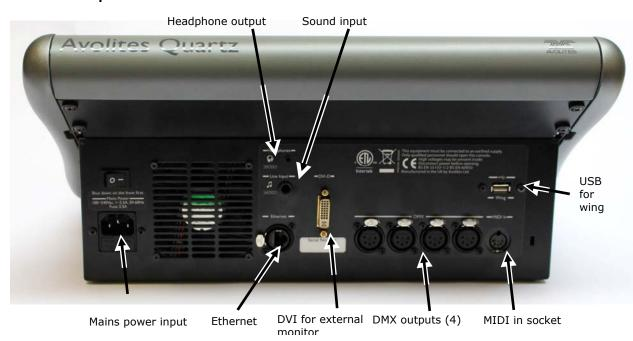
All the connections are on the rear panel. Most are self-explanatory. The power switch on the rear panel is an isolator for the power supply and should not be used to turn the console off. Use the switch on the front panel to turn the console on and off.
