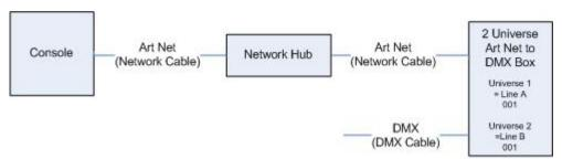
Using standard RJ45 ethernet cables, attach the devices together.
