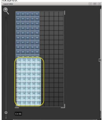
3> Drag the selected fixtures so they sit directly under the odd fixtures.
