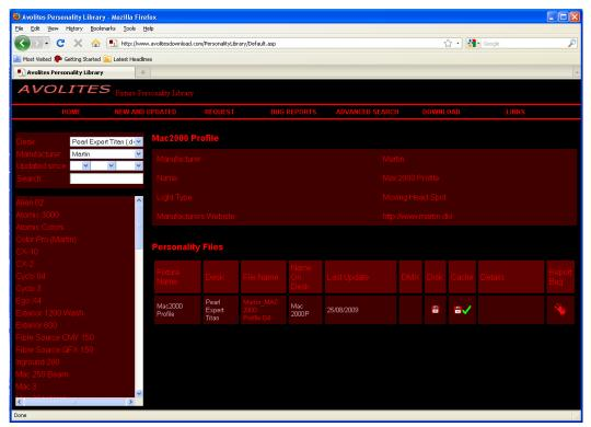
All available fixture personalities are listed down the left side of the screen. You can use the boxes on the top left to filter the list to show fixtures from specific manufacturers, or fixtures available for a certain console, or to search for a specific fixture name.
