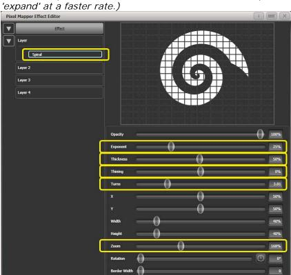
Increase 'Exponent' to around 25%. (This causes the spiral to 'expand' at a faster rate.)
