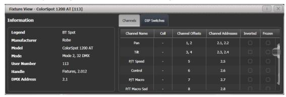
If the fixture address is set using DIP switches, the console can show you how to set the switches by clicking on the DIP Switches tab.
