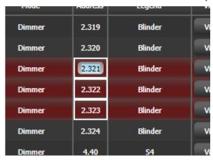
Type the new address for the first fixture in the selection and press Enter (using the format Universe . Address – if you miss out the universe part it will stay unchanged).
