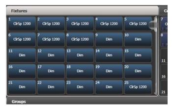
Fixture buttons can be shown either in pages with Page buttons, or you can use the scroll bar on the right to show different pages. Use the [Pages Show/Hide] button on the right of the screen to select between page buttons and scrolling mode. You can change the fixture page at any time.
