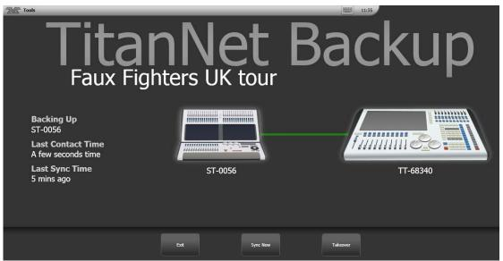
A green line between consoles represents a good connection. If a red line is shown there is a problem with the network connection. A blue line will appear during sync operations.
