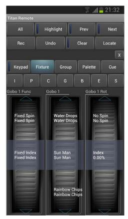
The wheels show function values (such as colours or gobo names). To go to the next function, just touch the arrows at the top or bottom of the wheel. To manually scroll the value, spin the wheel with your fingers. If there are more than three functions, touch the IPCGBES button again to change to the other functions.
