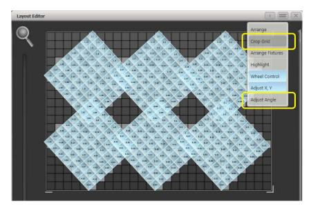
Note that underneath the visual representation of the fixtures the actual cells used are shown in light grey.
