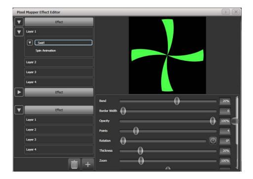
To see how the effect will look on the fixtures, open the Pixel Mapper preview window by pressing Window Open, [Open Workspace Window], [Pixel Mapper Preview]. A real life view of each effect running is shown in a button at the bottom of the screen, you can select each of these by pressing the button.
