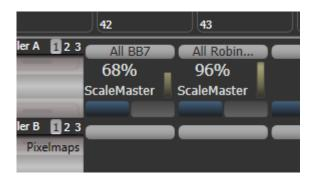
When a group master is set to disabled or moved to a handle without a fader, it will become locked at the current fader level.
